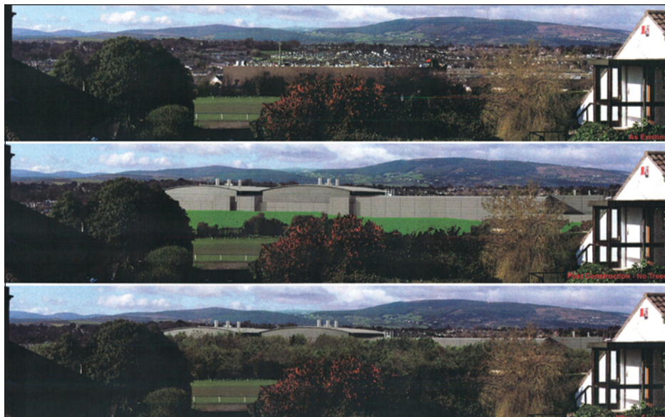
Primary neighbor elevation: the top photo shows the existing views, the middle photo shows the effect of the berms, and the bottom photo shows the final effect of the landscaped berm. Up to 14 of these composite images were developed and discussed with the neighbors for their feedback and agreement.
