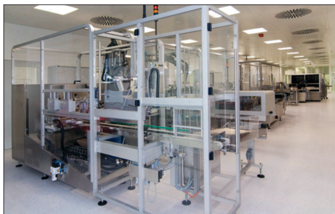
Pfizer Ireland Pharmaceuticals: in-line inspection machine.
